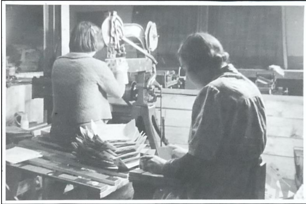
Workers at the General Paper and Box Manufacturing Company reinforcing the corners of pre-folded boxes.
